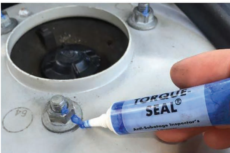
Torque Best Practice — Use Torque Seal to verify at a later time/date that you have completed the application of torque to the fastener.
