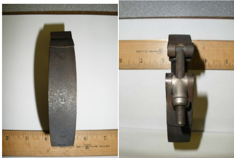
Figure 24 Spot-welded, 3-segment, Coupling
