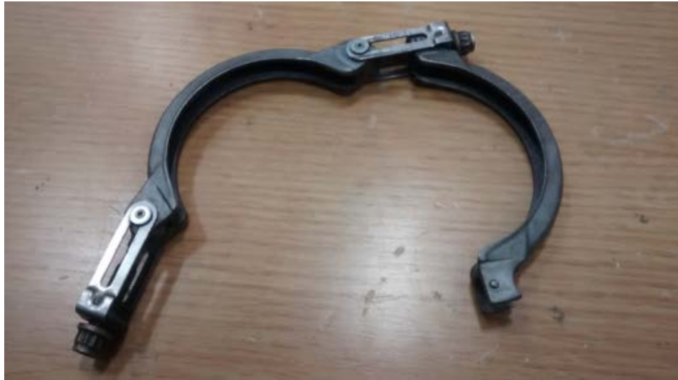
Figure 20 Forged and Machined Coupling
