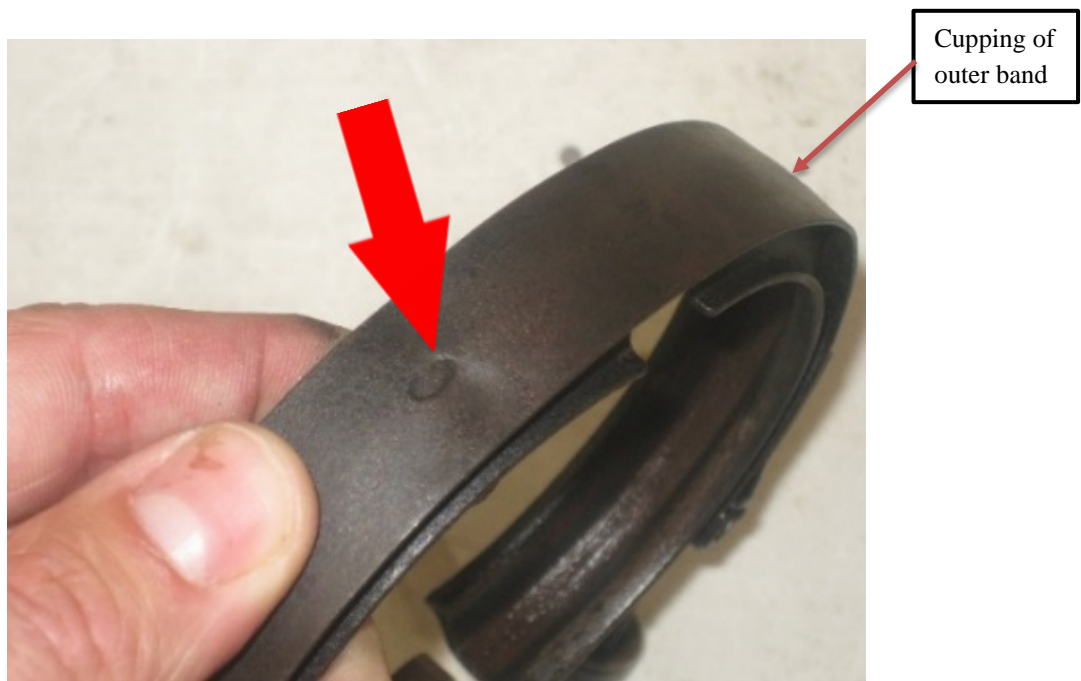
Figure 22 Spot-welded, 3-segment Coupling
