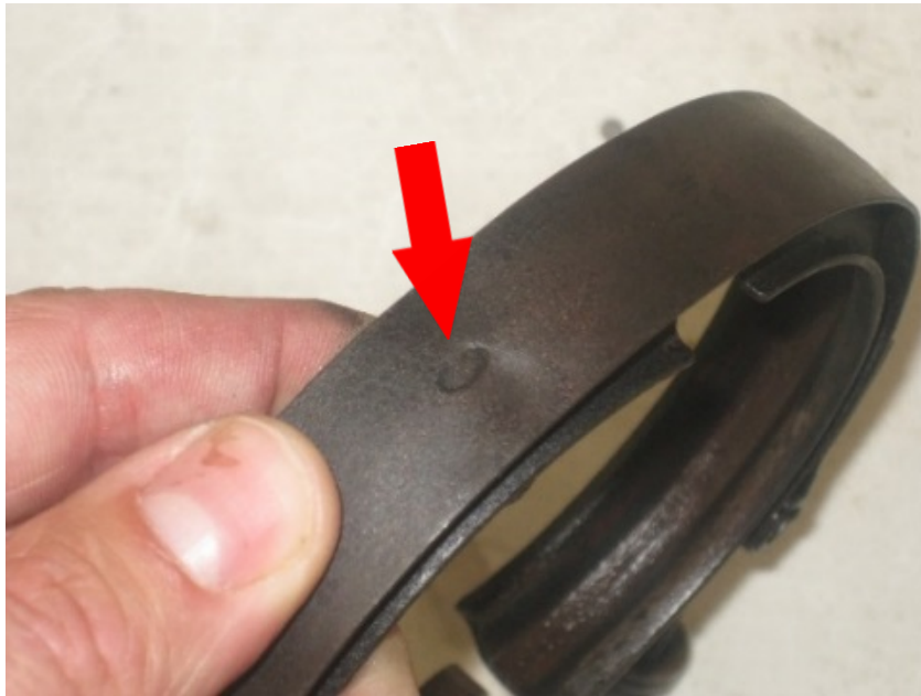
Figure 12 Spot-welded, 3-segment Coupling
