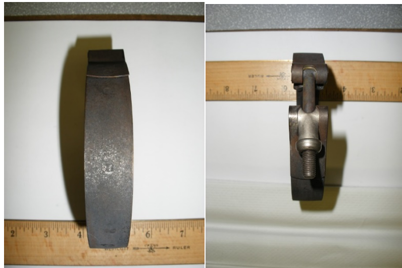
Figure 14 Spot-welded, 3-segment Coupling
